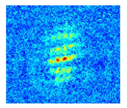
An example of an interference pattern produced by the atom interferometer Credit: ©: Maike Lachmann, IQO
