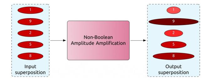
New amplification algorithms expand the utility of quantum computers to handle non-Boolean scenarios, allowing for an extended range of values to characterize individual records, such as the scores assigned to each disk in the output superposition above. Credit: Prasanth Shyamsundar
