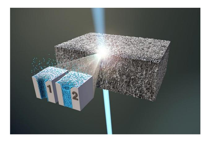
From the measurement data, the team was able to determine that the xenon atoms first accumulate on the inner walls of the pores (state 1), before they fill them up (state 2). The X-ray beam penetrates the sample from below. Credit: M. Künsting/HZB
