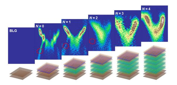
Using ultraviolet light, researchers probed the electronic characteristics of a 2D semiconductor (purple) as the number of substrate layers (green) increased. In the data maps, red circles mark an electronic feature that diminished as substrate layers were added. Credit: Meng Kai Lin/University of Illinois at Urbana-Champaign
