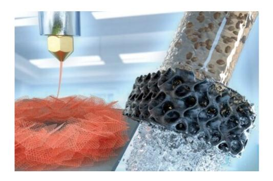
At left, a 3D printer printing the hexagonal-shaped graphene aerogel sheet. At the right, the aerogel (now black) filters dirty water. Credit: Environmental Science: Nano
