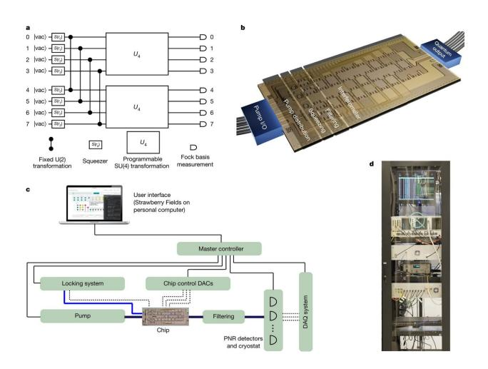
Overview of apparatus. a, Equivalent quantum circuit diagram illustrating the functionality of the photonic hardware. Up to eight modes initialized as vacuum are squeezed with squeezing parameters rk and entangled (via the fixed two-mode unitary transformation U(2) equivalent to a 50/50 beam splitter with the
