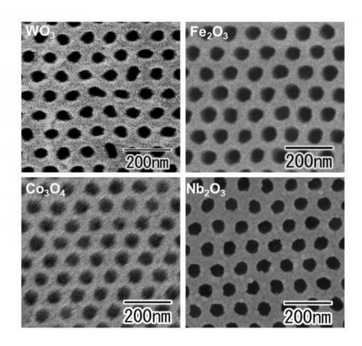
Scanning electron microscopy images of newly fabricated highly ordered nanohole arrays in tungsten, iron, cobalt and niobium oxide layers. Credit: Tokyo Metropolitan University
