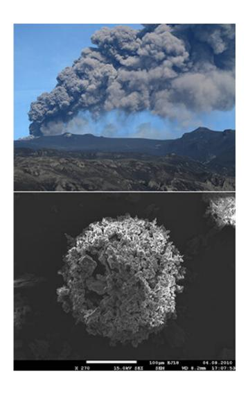
Volcanic plume associated with the April-May 2010 eruption of Eyjafjallajökull volcano (Iceland) and Scanning Electron Microscope image of a typical ash cluster made of micrometric volcanic particles collected on an adhesive paper during fallout. Credit: UNIGE, Costanza Bonadonna
