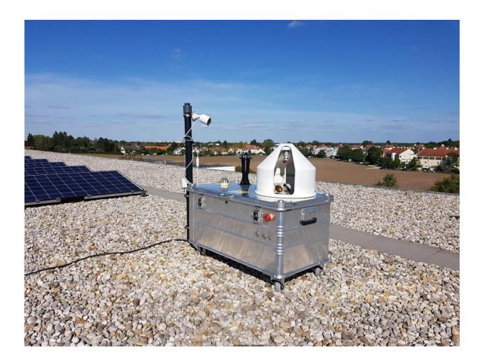
Measuring device of the MUCCnet sensor network set up by Prof. Jia Chen, Chair of Environmental Sensing and Modeling, at the TUM Department of Electrical and Computer Engineering of the Technical University of Munich (TUM) on the roof of a building in Taufkirchen. Credit: F. Dietrich/TUM
