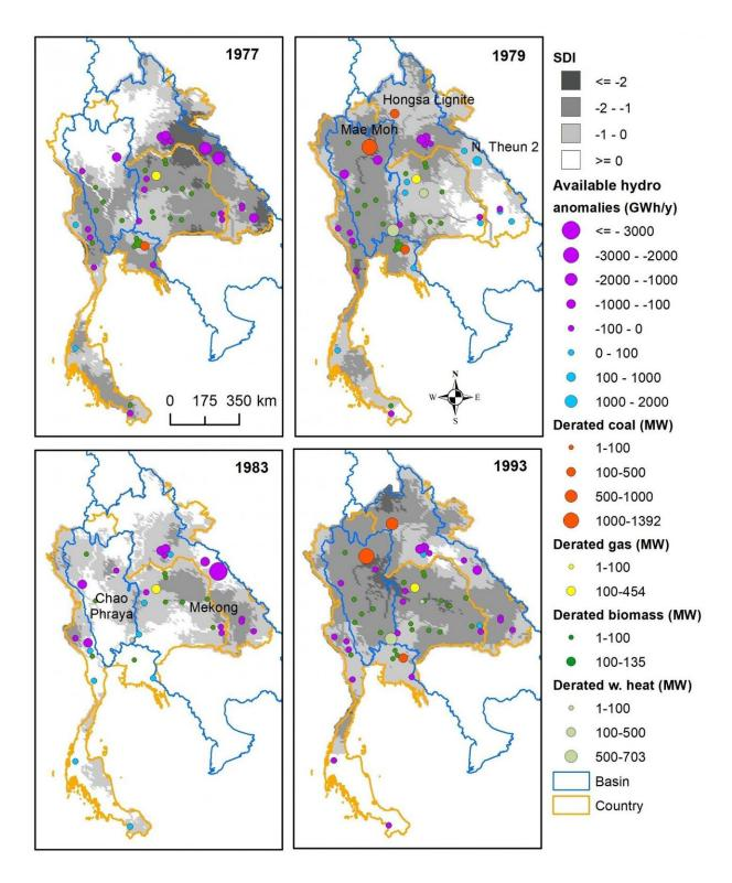
The figure illustrates the response of the Thai-Laotian power grid, built and operated in 2016, under the hydro-climatological conditions experienced in four selected years. The intensity of droughts across the Mekong and Chao Phraya
