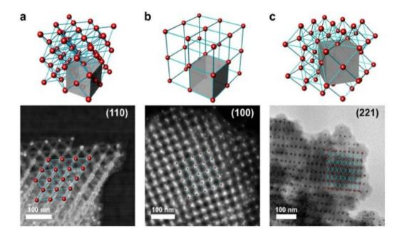
Different types of nanoscale lattices formed with polyhedra DNA nano-frames (tetrahedra, cubes, and octahedra) and gold nanoparticle are mineralized with controllable silica coating thicknesses (from about 5nm to a full space-filling). Credit: Oleg Gang/Columbia Engineering
