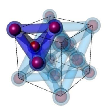
Mineralization of 3D lattice formed by DNA tetrahedra (about 30 nm) and gold nanoparticle into all-inorganic 3D silica-Au replicas with preserved architecture. Credit: Oleg Gang/Columbia Engineering
