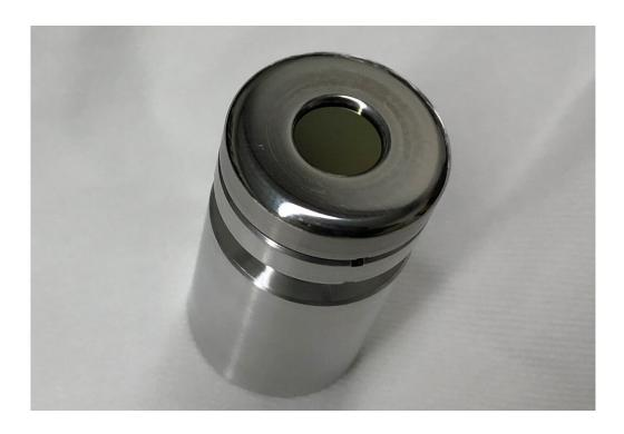
The full nitrogen-doped UNCD photocathode assembly tested on the Argonne Cathode Test Stand beamline. The nitrogen-doped UNCD sample is the dark central piece in the image. Credit: Jiahang Shao/Argonne National Laboratory
