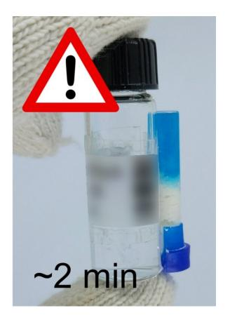
When the temperature of a glass vial containing simulated vaccine rises above -60 C for longer than 2 minutes, a blue dye in an adjacent tube diffuses into a white absorbent, leaving an irreversible color trace. Credit: Adapted from ACS Omega 2021
