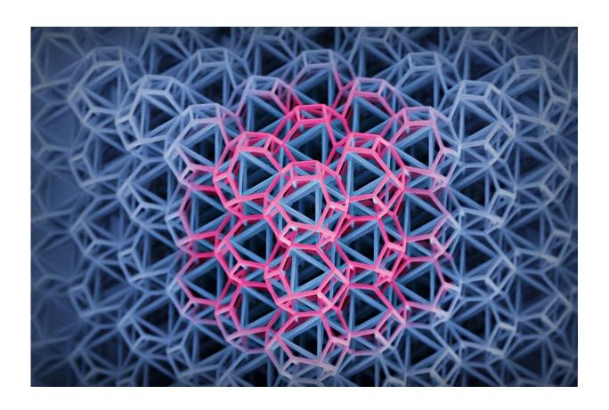
Novel tensegrity metamaterials by UCI and Georgia Institute of Technology researchers employ isolated compressive loop elements that are exclusively connected through a continuous network of tensile members (highlighted in magenta). Credit: Jens Bauer and Cameron Crook / UCI
