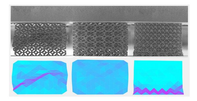
In a comparison with two other state-of-the-art nanoscale structures, the tensegrity lattice created by UCI and Georgia Tech researchers (center) exhibited a 25-fold improvement in deformability and an orders-of-magnitude increase in energy absorption. Credit: Jens Bauer and Cameron Crook / UCI
