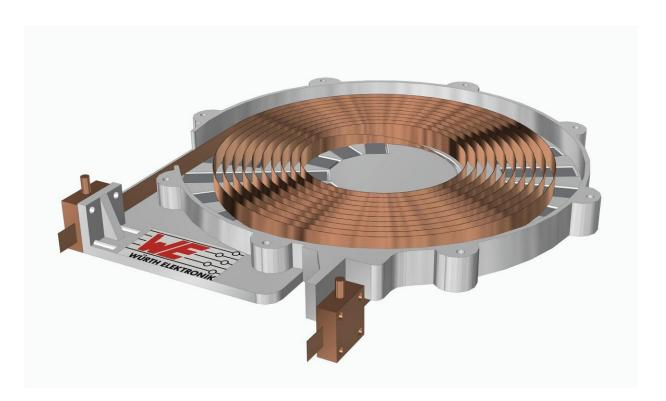
A team of physicists at the Technical University of Munich has developed a coil made of superconducting wires that can transmit power of more than five kilowatts contactless without major losses. Credit: Christoph Utschick / Wuerth Elektronik eiSos
