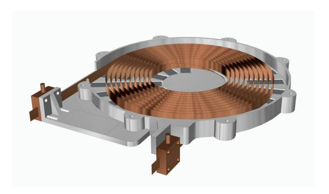
A team of physicists at the Technical University of Munich has developed a coil made of superconducting wires that can transmit power of more than five kilowatts contactless without major losses. Credit: Christoph Utschick / Würth Elektronik eiSos
