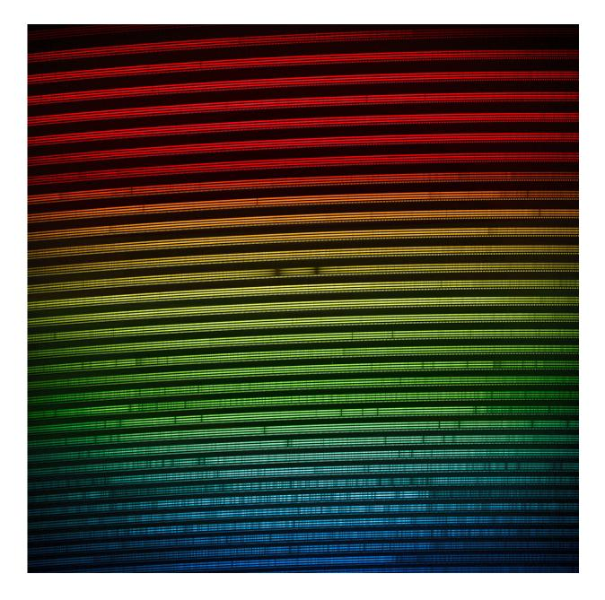
Colorized 2D spectra of the star Gliese 486 as seen with MAROON-X. The two spectra are from the two camera arms of MAROON-X. Each spectrum covers the 500-670 nm wavelength range and the color-coding corresponds to how a human eye would perceive the colors. Credit: International Gemini Observatory/NOIRLab/NSF/AURA/A. Seifahrt
