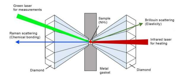
Schematic representation of the diamond anvil cell. The chemical structure can be determined with the Raman spectrum, and the elasticity of the sample material with Brillouin scattering. Credit: ETH Zurich / T. Kimura
