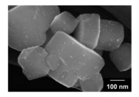
Pt-modified BaTaO2N photocatalysts. Credit: Cited from Wang, Z., Luo, Y., Hisatomi, T. et al. Sequential cocatalyst decoration on BaTaO2N towards highlyactive Z-scheme water splitting. Nat Commun 12, 1005 (2021). Copyright © 2021, The Authors.
