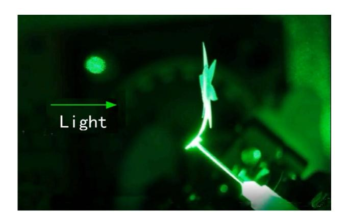
Photonic material in the shape of a flower can move in response to light, closely tracking the angle of maximum exposure. Credit: Fio Omenetto, Tufts University
