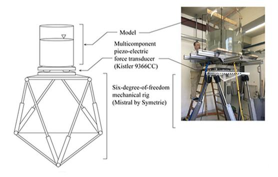
A study using a scale-model fish containment system is reported in *Physics of Fluids* and shows why violent sloshing motions, which endanger cages and fish, arise and how to minimize them. This image shows the scale-model fish tank with mechanical rig to create sloshing. Credit: Claudio Lugni
