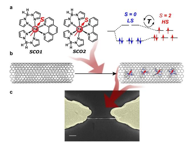
Iron-based SCO molecules encapsulated in a single carbon nanotube. Credit: Nature Communications
