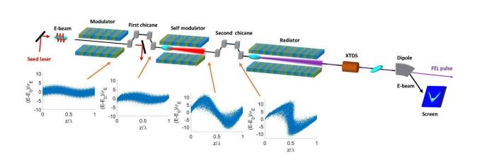
The self-modulation scheme together with the electron-beam longitudinal phase spaces at various positions. Credit: SARI
