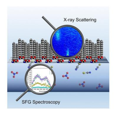
Scientists used X-ray scattering techniques (top) and sum frequency generation spectroscopy (bottom) to study the separation mechanisms at the interface of water and oil (depicted here) during extraction. Credit: Argonne National Laboratory
