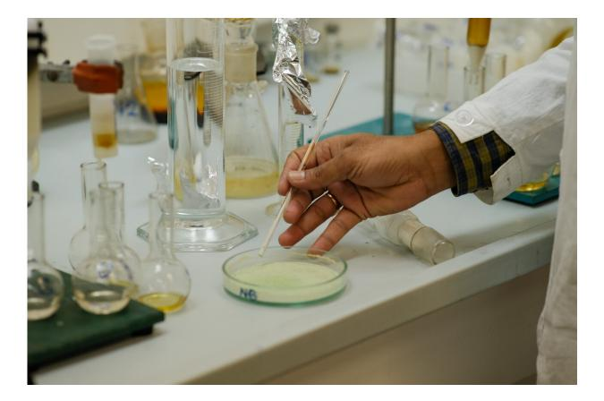
A film of ferulic acid and sodium alginate formed on the surface of the glass Petri dish. Credit: UrFU / Andrei Fomin
