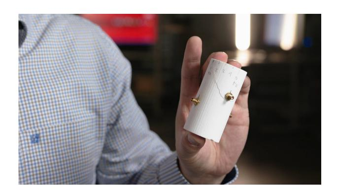
Sandia National Laboratories geoscientist Hongkyu Yoon holds a fractured 3D-printed rock. Hongkyu squeezed 3D-printed rocks until they cracked and listened to the sound of the rocks breaking to be able to identify early signs of earthquakes. Credit: Rebecca Gustaf
