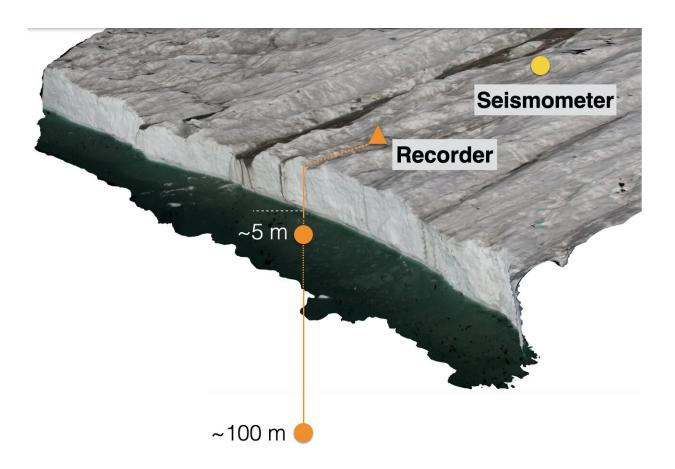
The model of the study site in July 2017, showing the positions of the sensors at different locations and depths. Credit: Evgeny A. Podolskiy
