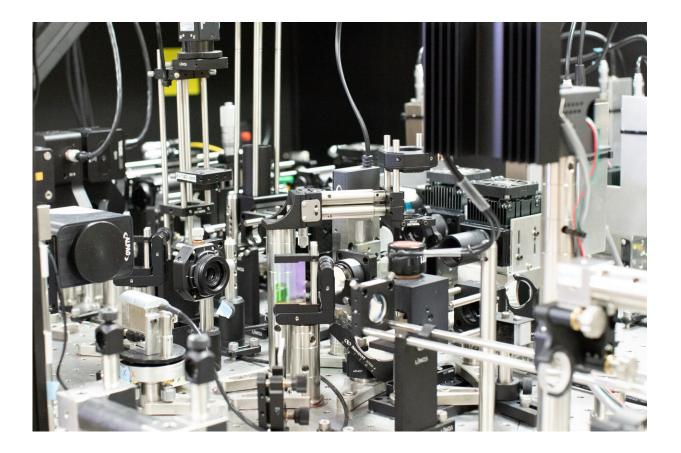
The researchers customized this adaptive optics scanning light ophthalmoscope to improve the imaging resolution by strategically blocking light in various locations of the instrument. Using less light is an advantage for imaging the human eye. Credit: Johnny Tam, National Eye Institute
