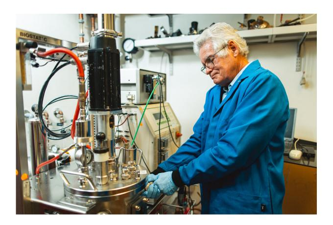
James Swartz operating a bioreactor that his lab uses to grow cells from which cell extracts used for CFPS are prepared. Credit: Andrew Brodhead
