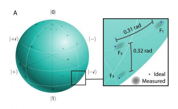
Each point on the sphere of this visual representation of arbitrary frequency-bin qubit states corresponds to a unique quantum state, and the gray sections represent the measurement results. The zoomed-in view illustrates examples of three quantum states plotted next to their ideal targets (blue dots). Credit: Joseph Lukens and Adam Malin/ORNL, U.S. Dept. of Energy
