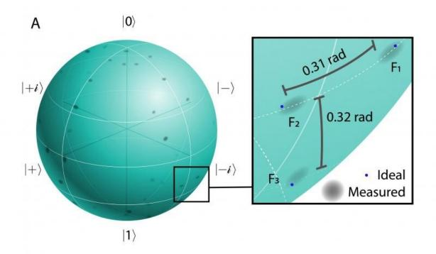
Each point on the sphere of this visual representation of arbitrary frequency-bin qubit states corresponds to a unique quantum state, and the gray sections represent the measurement results. The zoomed-in view illustrates examples of three quantum states plotted next to their ideal targets (blue dots). Credit: Joseph Lukens and Adam Malin/ORNL, U.S. Dept. of Energy
