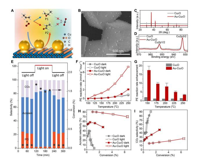
Characterization of Au-Cu2O catalyst and its catalytic performance response to illumination. (A) Schematic of the SP-regulated partial oxidation of propylene
