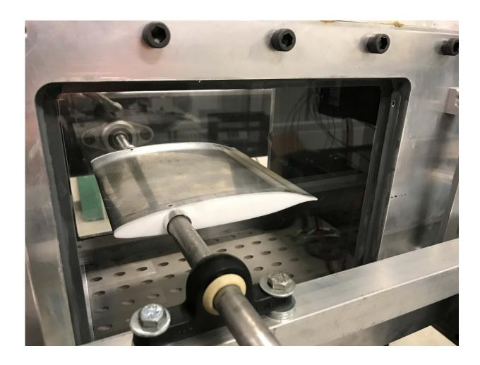
Griffith-type transonic airfoil inside the wind tunnel test section. Credit: University of Illinois Urbana-Champaign
