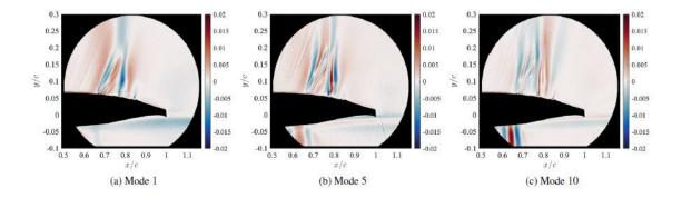
Three modes showing Mach wave build up leading to fully developed shock, oscillation, and dissipation. Credit: University of Illinois Urbana-Champaign
