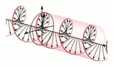
A schematic of circularly polarized light. Photons that move in unison along a spiral path, rather than a conventional wave pattern, produce circular polarized light. The light-emitting perovskite layer of the spin-LED device produces either left-handed or right-handed polarized light, depending the spin of the electrons that made it past the perovskite filter. Credit: Dave3457 via Wikicommons
