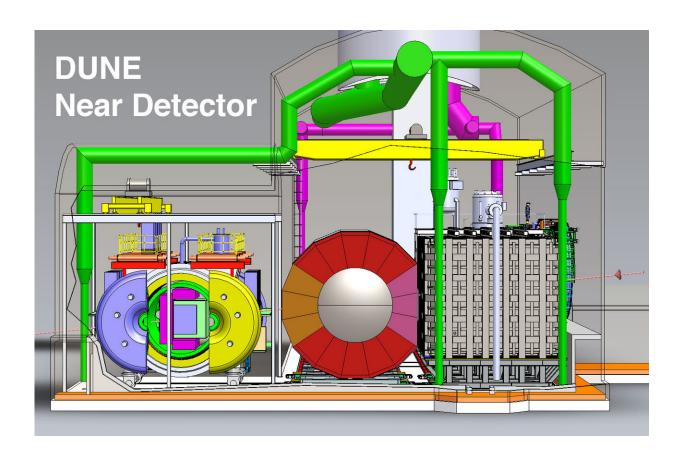
One of the DUNE near detector's subdetectors, SAND, will detect neutrinos with an electronic calorimeter, which measures particle energy, and a tracker, which records particle momenta and charge. A second subdetector will use liquid argon to mimic the neutrino interactions in the far detector. The third will use gaseous argon. Working together, they will measure particles with more precision than other neutrino detectors have able been to achieve. Credit: DUNE collaboration
