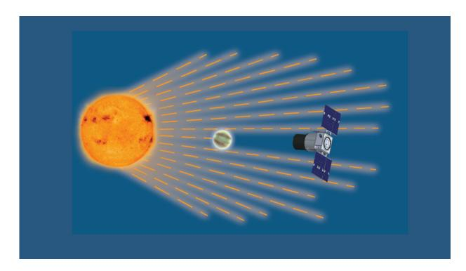
This illustration depicts Pandora's use of transit spectroscopy to reliably identify an exoplanet's atmospheric composition as it passes in front of its host star. Credit: Lawrence Livermore National Laboratory and NASA's Goddard Space Flight Center
