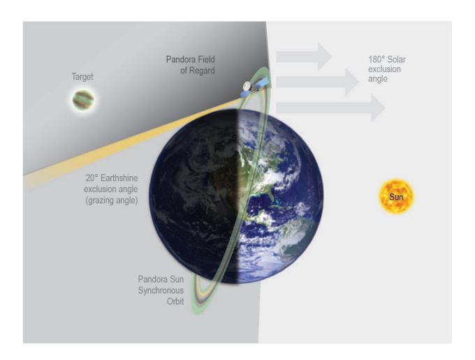
This illustration (not to scale) depicts Pandora's orbital pattern in Sunsynchronous low-Earth orbit, located approximately 435 to 497 miles (700 to 800 kilometers) above Earth's surface, as it observes its targeted exoplanets and
