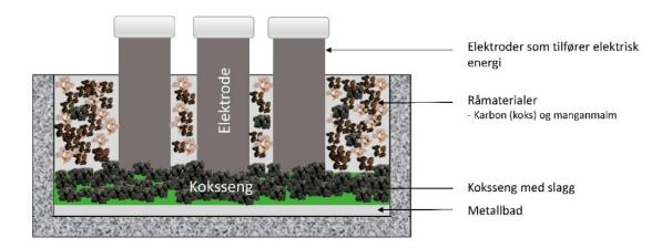
The illustration shows a furnace that produces manganese alloys. Credit: Trine Asklund Larssen, NTNU / SINTEF
