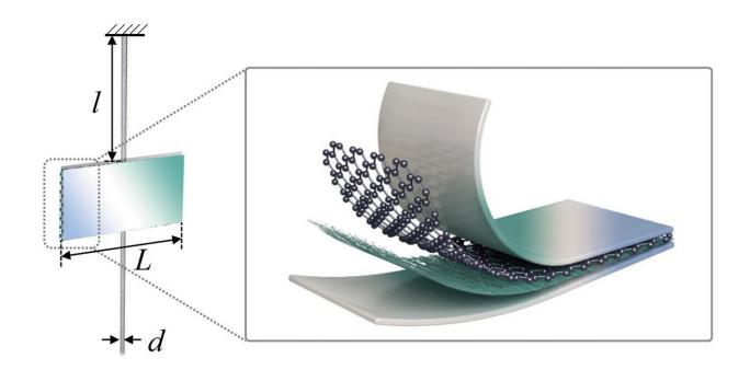
Schematic illustration of the torsion balance unit. It consists of an Al/graphene/CNT/Al mirror with beam length L suspended by an individual CNT with diameter d and suspension length l. Credit: Science Advances, doi: 10.1126/sciadv.abd2358
