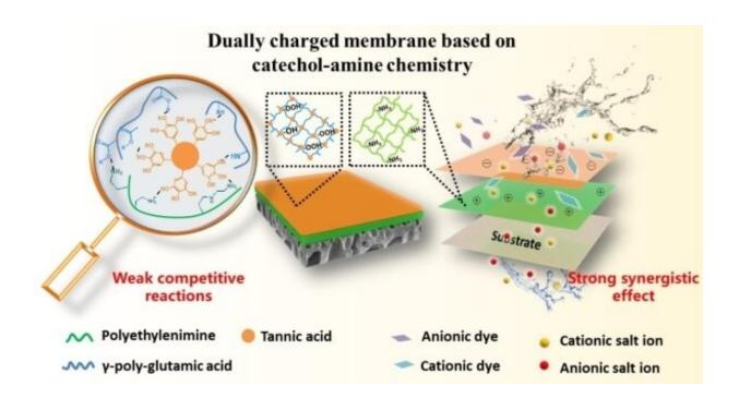
Diagram of the dually charged membrane fabricated via catechol-amine chemistry surface engineering. Credit: CAO Yang
