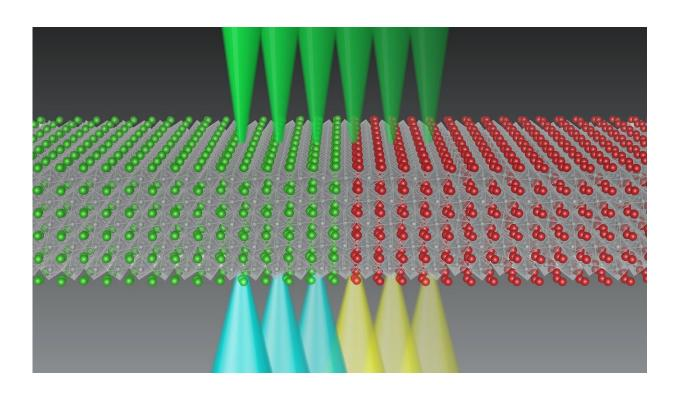
Schematic illustration of a STEM probe scanning across the interface of two nickelate compounds, with the nature of the scattered electrons changing as the electronic phase of the material goes from being metallic to insulating. Image credit: Duncan T.L. Alexander. Atomic structure model rendered using VESTA. Credit: Ecole Polytechnique Federale de Lausanne (EPFL)
