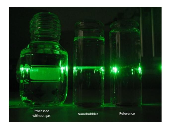
Sample in the middle scatters coherent laser light which indicates presence of nanosized bubbles. Scattering of the laser light indicates presence of surfaces. In daylight, all samples are transparent which presents that the surfaces are in nanoscale. Credit: Tapio Vehmas
