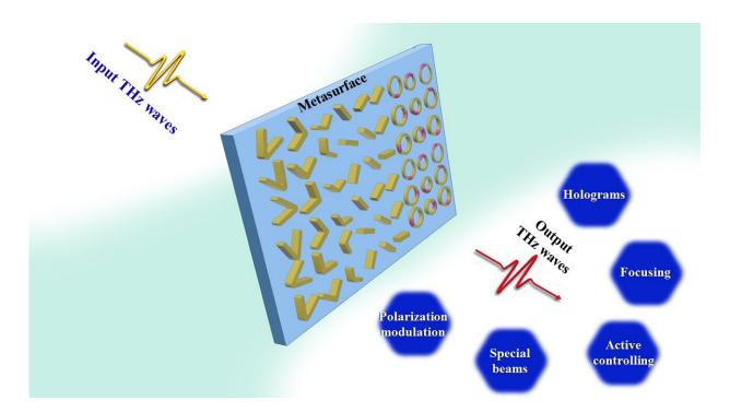
The associated THz responses include focusing, holograms, polarization modulation, special beams and active controlling. Credit: Xiaofei Zang, Bingshuang Yao, Lin Chen, Jingya Xie, Xuguang Guo, Alexei V. Balakin, Alexander P. Shkurinov, and Songlin Zhuang
