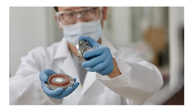
Dehumidifiers with enhanced polyimide membranes (white disc) will be energy efficient with a smaller carbon footprint. Credit: Dharmesh Patel/Texas A&M Engineering
