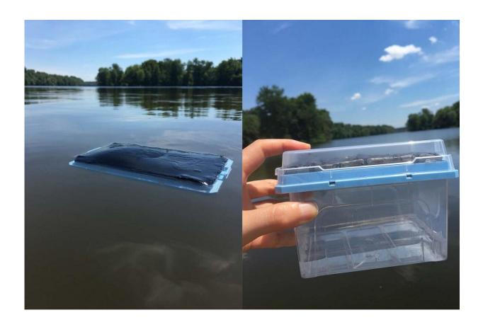
In a study conducted at Princeton University, researchers placed the gel in lake water where it absorbed pure water, leaving contaminants behind. The researchers then placed the gel in the sun, where solar energy heated up the gel, causing the discharge of the pure water into the container. Credit: Xiaohui Xu, Princeton University
