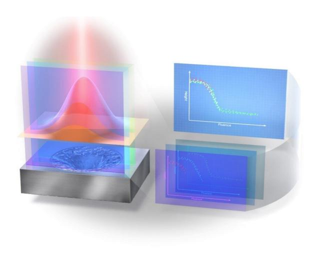
(Lower left) The laser makes a hole in a material. (Upper left) The fluence of the laser is measured. (Lower right) Measurements of the fluence and the hole depth are superimposed. (Upper right) The relationship between these measurements is then determined so that hole depth can be calculated based solely on the fluence. Credit: © 2021 Sakurai et al.
