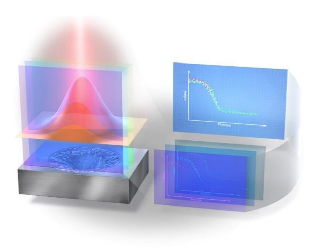
(Lower left) The laser makes a hole in a material. (Upper left) The fluence of the laser is measured. (Lower right) Measurements of the fluence and the hole depth are superimposed. (Upper right) The relationship between these measurements is then determined so that hole depth can be calculated based solely on the fluence. Credit: © 2021 Sakurai et al.
