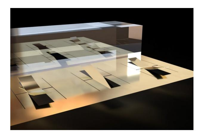
Strategically placed cuts to structural films can create 3D nanostructures when force is applied to the films, similar to how kirigami cuts made to paper can create pop-up structures. Credit: Jennifer M. McCann/Penn State MRI
