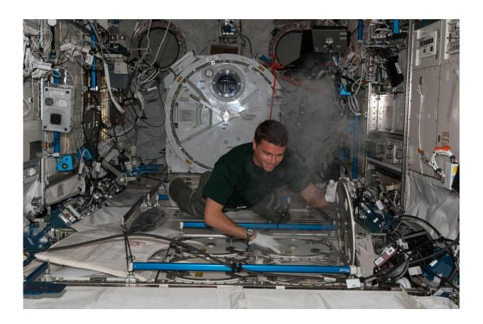
NASA astronaut Reid Wiseman inserting human biological samples in the Minus Eighty Laboratory Freezer for ISS (MELFI). Archived data from these samples later were used by researchers studying the effects of space on the immune system. Credit: NASA
