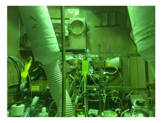
Pm-147, a high-demand isotope that is used in nuclear batteries, is isolated from other byproducts of Pu-238 production in hot cells in ORNL's REDC before it's purified and readied to ship to customers. Credit: Richard Mayes/ORNL, U.S. Dept. of Energy
