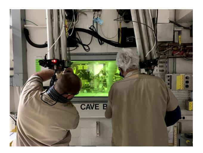
Technicians John Dyer and T. Dyer use a manipulator arm in a shielded cave in ORNL's Radiochemical Engineering Development Center to separate concentrated Pm-147 from byproducts generated through the production of Pu-238. Credit: Richard Mayes/ORNL, U.S. Dept. of Energy
