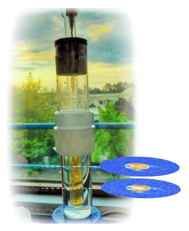
The phantom used for hyperpolarized imaging, with an illustration of imaging slices acquired using the new technique. Credit: ©: Laurynas Dagys, University of Southampton
