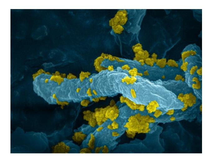
D. desulfuricans-CdS hybrids display high H2 production activity, high stability and a remarkable efficiency in the direct use of solar energy. Credit: Inês Cardoso Pereira; Mónica Martins
