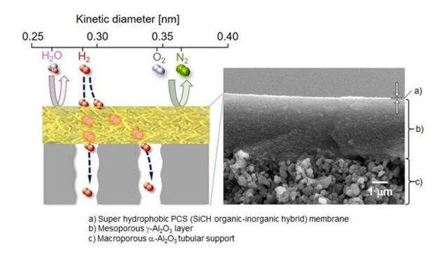
A cross-sectional image of selective hydrogen gas permeation in a super hydrophobic membrane formed on a porous tubular support. Credit: Yuji Iwamoto from Nagoya Institute of Technology
