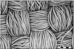
Scanning electron microscope images of cotton flannel (left) and polyester (right). Cotton fibers absorb moisture from breath, which increases filtration. Each segment of the image scale bars is 50 micrometers, or millionths of a meter -- roughly the width of a human hair. Credit: E.P. Vicenzi/Smithsonian's Museum Conservation Institute and NIST
